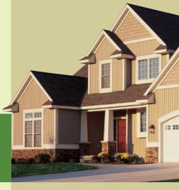
Vinyl siding, unlike some other exterior cladding, provides exceptional rainscreening performance. It effectively enables moisture to drain out of an exterior wall assembly, dramatically reducing water accumulation that can lead to rot and mold.
