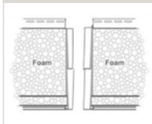
FIGURE 1 - Use factory notches (rear view)
